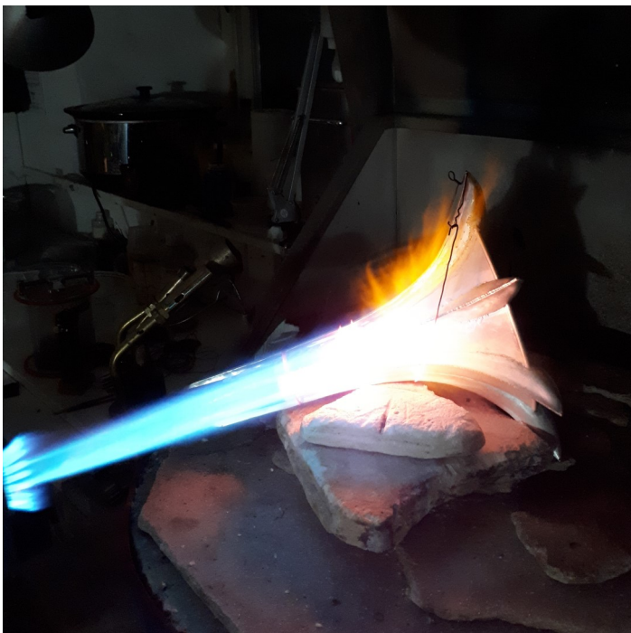
Soldering the top of one of the Acolyte Candles. Courtesy Rauni Higson
