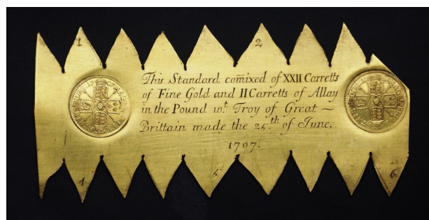
The 1707 trial plate for 22 carat gold. The two die impressions are both the reverse of a Queen Anne 1707 two guineas. Courtesy The Royal Mint
